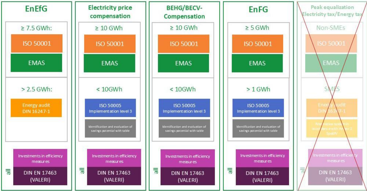
Figure 3: based on Prof Dr Ulrich Nissen - Integration of standards (ISO 50001, DIN 16247-1, DIN 17463, EMAS) into legal requirements
